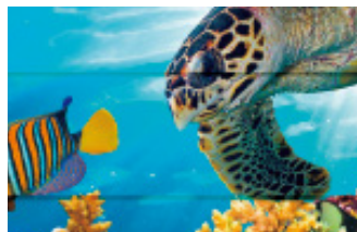
Overlap/Black streaks (Insufficient feeding amount)
