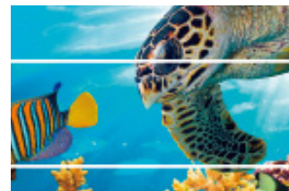
Gap/White streaks (Excessive feeding amount)
