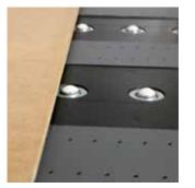
The Jeti Tauro ABF **vacuum belts** are perfectly aligned at all times, feeding media smoothly into the engine. Several release rollers at the back of the table support this feeding process. While one board is being printed, the front vacuum belts are switched off to allow loading of the next board.
